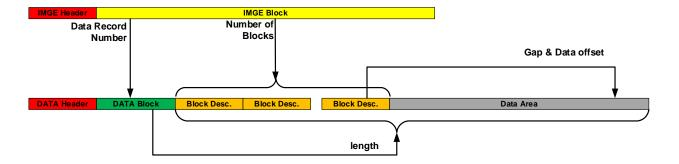
The overall size of an IMGE record is 80 bytes (12 for the header block and 68 for the IMGE block).
