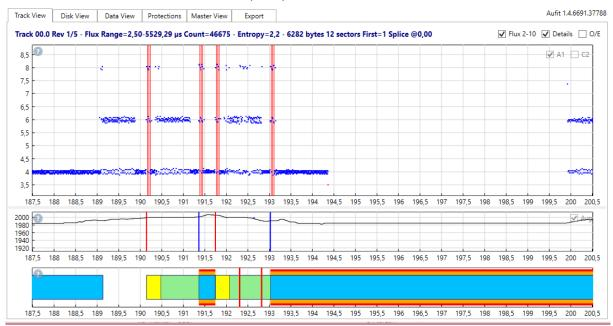
Here we can see that around the position 194500µs till almost 200000µs (the end of track) there are **no flux transitions**. This NFA is directly located at the end of the track inside the sector 11 and 12. This alone explains why these two sectors read with fuzzy bits due to multiple timing errors.
